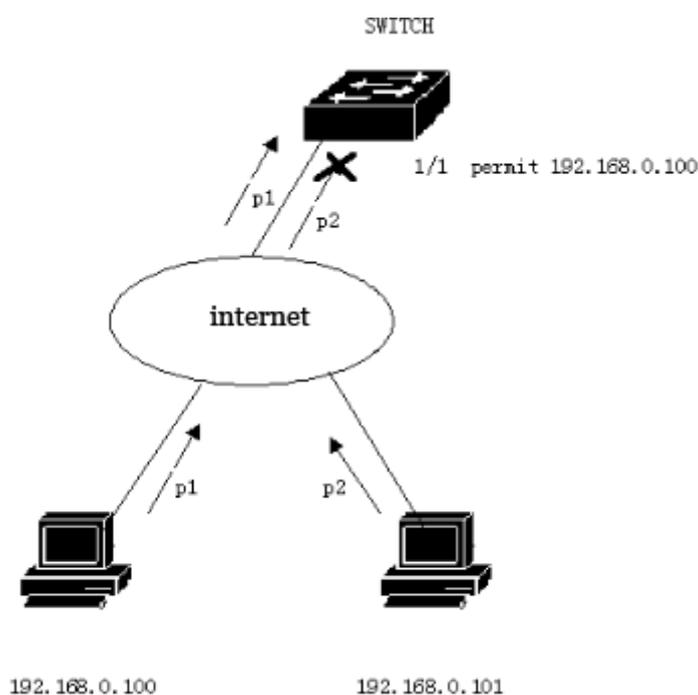
When multiple ports are used for ACL filtering, the same ACL rule group can be used, and the same filtering rules are used.
