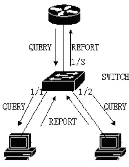
As shown in Figure 1, host 1 has added multicast group ff15:: 1, and now host 2 wants to join multicast group ff15:: 1. When the host 2 received MLD QUERY packet after sending back a MLD REPORT packet switch MLD REPORT received from the 1/2 port will put the package from the 1/3 port and forwarded the query packet port 1/2 was added to the two layer multicast entry, the entry into the two layer multicast:
