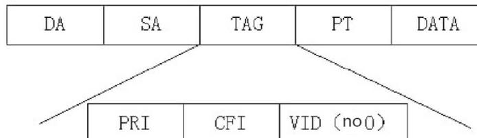
All data frames within a switch are marked. If a marker free data frame is entered into the switch, the switch adds a tag to the data frame, and selects a VLAN ID value to fill in the marked VID. If a data frame with VID 0 is entered into the switch, the switch selects a VLAN ID value to fill in the marked VID. If a data frame with VID non 0 tag is input to the switch, the frame remains unchanged.
