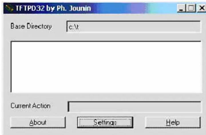
Then: Setting the TFTP Server file directory. After you start TFTP Server, reset the TFTP Server file directory and copy the image files that you want to load into this directory. The specific operation is, click the [Settings] button, there TFTP32 settings interface, as shown below.
