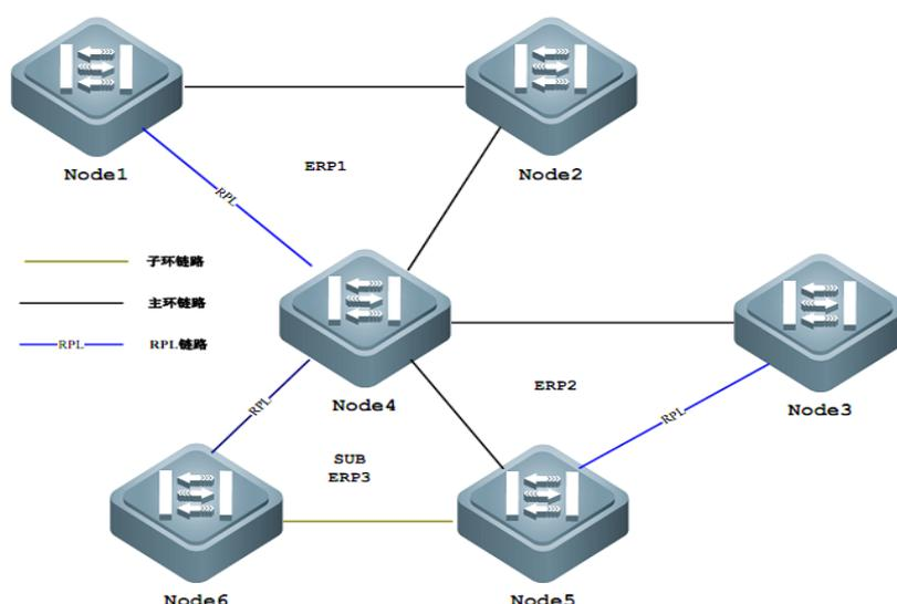
As shown in the figure above, ERPS supports the addition of multiple rings in the same node (Node4) as tangent or intersection, greatly increasing the flexibility of networking.
