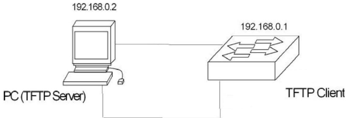
The configuration port of the switch is connected to a configuration terminal through the cable and connected with a PC through the network cable. Install TFTP Server in PC, configure Ethernet port IP address of PC, assume the IP address of PC is 192. 168.0.2. Then, configure the IP address of the switch, where the IP address of the switch is assumed to be 192.168. 0.1 to ensure the connectivity between the PC and the switch.
