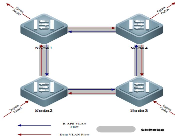
There are two types of ERPS in VLAN, one is RAPS VLAN, and the other is data VLAN. RAPS VLAN is only used for transmitting ERPS protocol packets; ERPS also only deals with protocol packets from RAPS VLAN, does not handle any protocol attack packets from data VLAN, and improves the security of ERPS.
