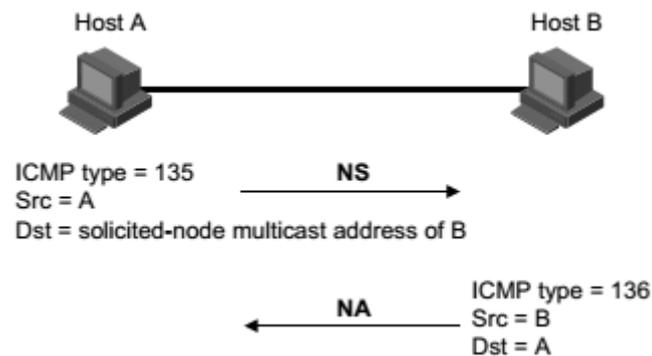
Schematic diagram of address resolution in Figure 1-3
