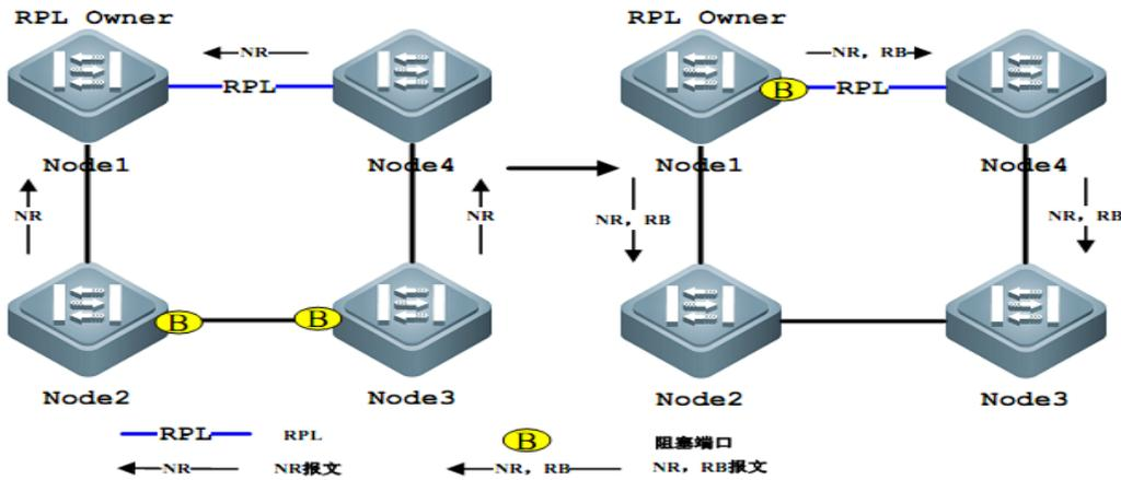
(1) When the fault is resumed, the neighboring nodes of the fault continue to block and send RAPS (NR) messages to indicate that there is no local fault;
