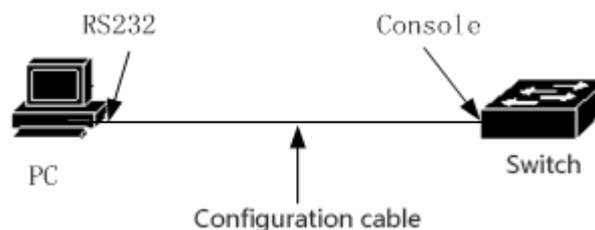
Second steps: Start the terminal emulation program on the PC machine (such as the super terminal of Windows), Configuring communication parameters of terminal emulation program.
