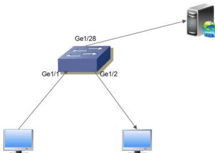
Configure VLAN, start global IGMP snooping, configure MVR VLAN, MVR program group range, global enable MVR:
