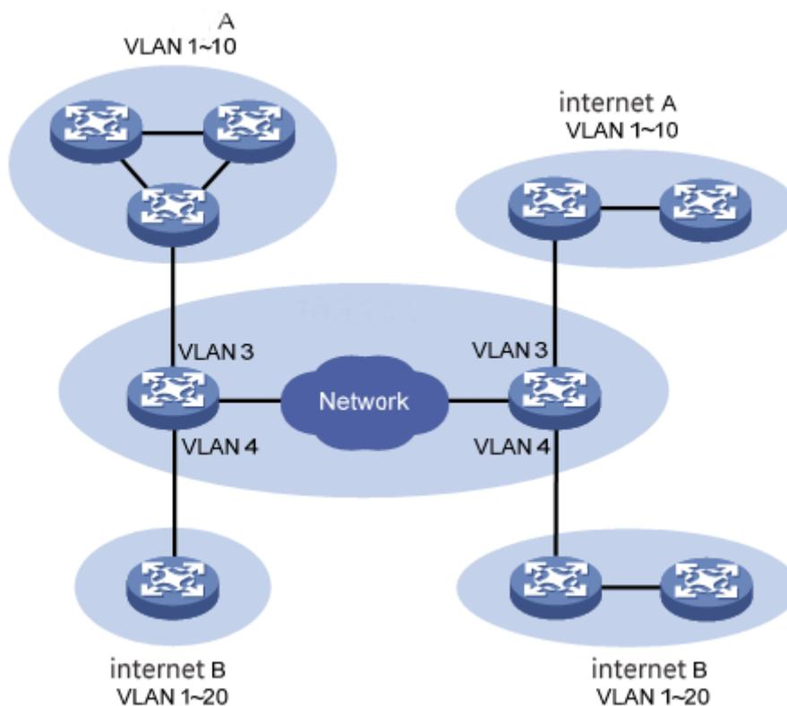
QinQ features enable the network to provide 4094X4094 VLAN at most, and meet the requirement of VLAN in metropolitan area network, It mainly solves the following problems:
