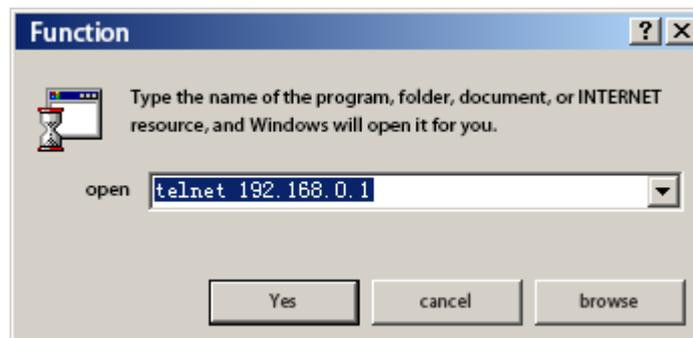
Fourth steps: If the system does not have a password, the Telnet interface goes directly to the CLI, and the CLI prompt appears (default is Switch >).; If the system sets the password, you need to enter the password on the Telnet interface to enter the CLI.
