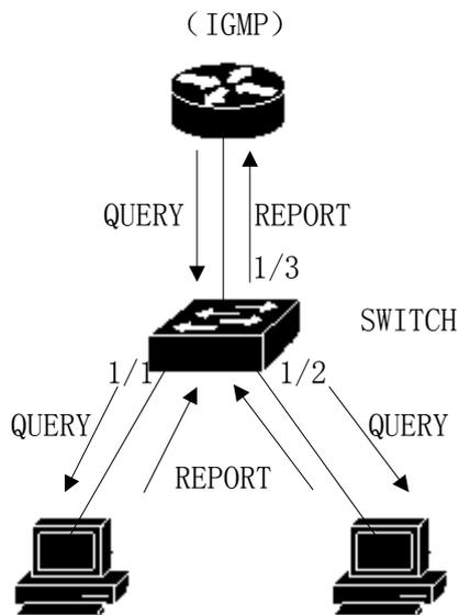
As shown in Figure 1, host 1 has added multicast group 224.1.1.1, and now host 2 wants to join multicast group 224.1.1.1. When the host 2 received IGMP QUERY packet after sending back a IGMP REPORT packet switch IGMP REPORT received from the 1/2 port will put the package from the 1/3 query port forwarded and make port 1/2 was added to the two layer multicast entry, the entry into the two layer multicast :
