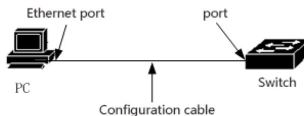
Second steps: Set the IP address of the Ethernet port of the PC machine, The IP address must be in the 192.168.0.0/24 segment (such as IP address 192.168.0.100)。 Judging the connectivity between PC and switch through Ping 192.168.0.1。
