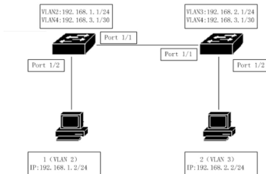
In the diagram, the switch 1 is a two layer switch, and the switch 2 is a three layer switch.
